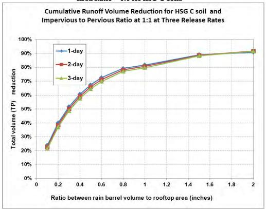
Figure 3- 37: Impervious Area Disconnection through Storage: Impervious Area to Pervious
