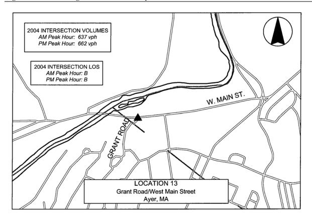
Approximately 650 vehicles were counted at this intersection for both the AM and PM peak hours. Intersection capacity analyses using the 2004 volumes were conducted for the AM and PM peak hour conditions. The intersection operates at LOS B during both the AM and PM peak hours.
