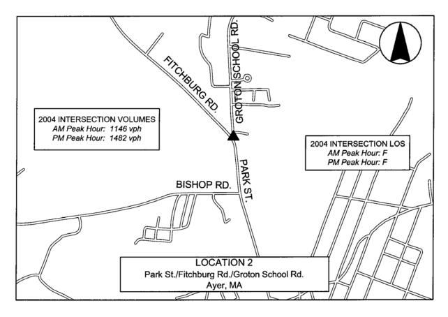
The Final EIR indicated that the signalization of this intersection was an existing (immediate) need due to the failure conditions identified for vehicles attempting to enter Route 2A (Park Street) from Route 111 (Groton School Road). This need was based upon 1990 peak hour traffic volumes.
