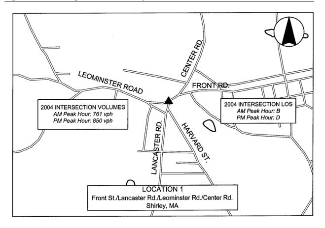
Traffic volumes and intersection Levels of Service (LOS) for the AM and PM peak hours are summarized in the above figure. Traffic volumes have increased by about 3% in the AM peak hour 8% in the PM peak hour over 2002 conditions. This location operates at LOS B during the AM peak hour, and LOS D during the PM peak hour.
