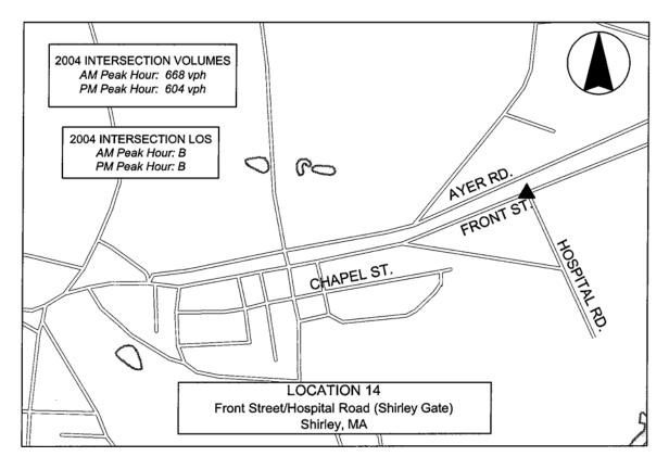
Over 600 vehicles were observed at this intersection during the AM and PM peak hours. Intersection capacity analyses using the 2004 volumes were conducted for the AM and PM peak hour conditions. The intersection operates at LOS B during both the AM and PM peak hours.
