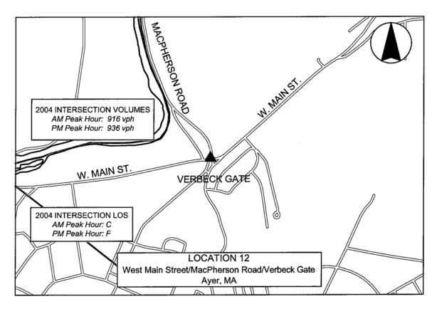
The year 2004 AM traffic volumes are about 100 vehicles lower than the year 2002 and about 20 vehicles lower than in the PM peak hour. Previous intersection capacity analyses indicated the need for signalization as a mid-range to long-range improvement as the build-out of Devens approaches. Intersection capacity analyses conducted for 2004 peak hour conditions indicate a LOS C conditions for the AM peak period and LOS F for the PM peak hour period.
